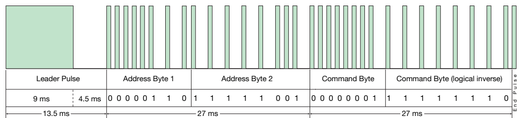
Figure 6-1. NEC Protocol Message Format
